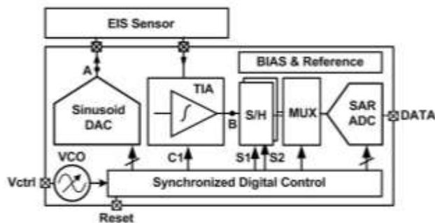
Fig. 2 Block diagram of the proposed EIS system.
