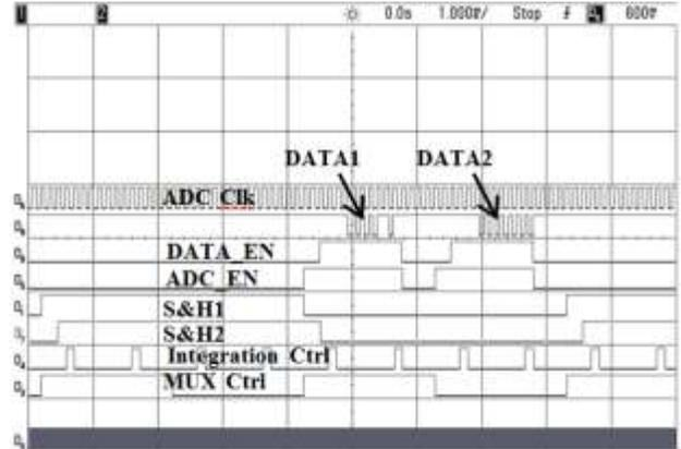
Fig.7 Measured clock and timing signal.
