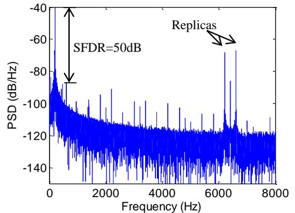
Fig.9: FFT of generated 1KHz sinusoid.
