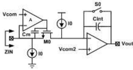
Fig. 5 The proposed EIS detection circuit.
