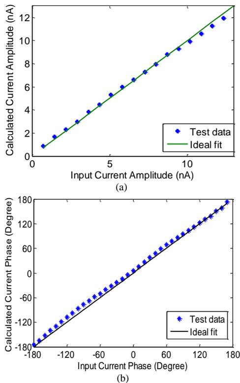
Fig. 10: Proposed detection function test with ideal sinusoid current with a) Fixed phase and sweep amplitude; b) Fixed amplitude and sweep phase.
