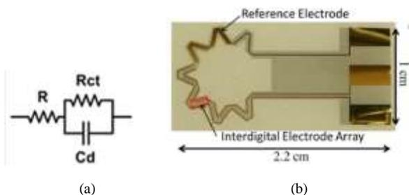
Fig. 1 (a) Simplified equivalent circuit for EIS; (b) EIS sensor.
