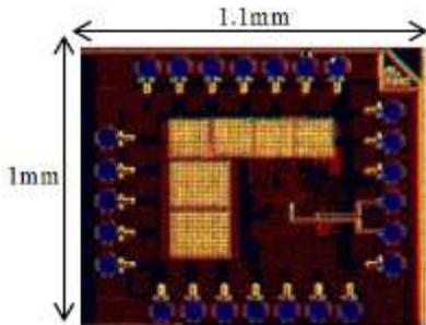
Fig. 6: Die photo of the EIS chip
