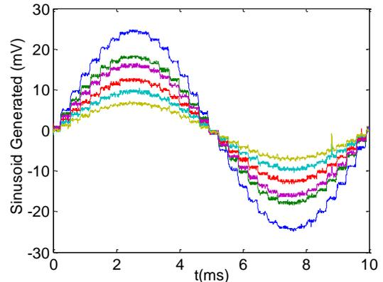
Fig. 8: Sinusoid DAC output cross amplitude setting.
