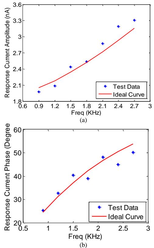
Fig. 11: System test data with on-board circuit model of sensor: (a) target conductance (impedance) amplitude change according to frequency sweep; (b) target conductance phase change according to frequency sweep.
