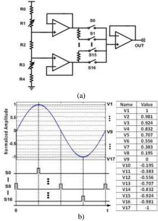
Fig. 4 The proposed sinusoid DAC: a) basic structure; b) digital control and reference selection.
