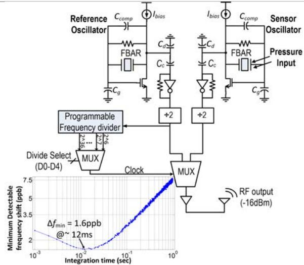
Figure 27.4.2: System block diagram and oscillator circuitry with Allan deviation measurements.
