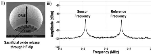
Figure 27.4.3: i, ii) SEM of the FBAR-CMOS die with the etch hole. iii) Sensor output (max hold on a spectrum analyzer) at a distance of 2m.
