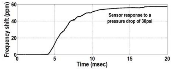
Figure 27.4.4: Sensor calibration curve from 20-70psi and time domain response of sensor simulating a tire blowout (pressure drop of 30psi).
