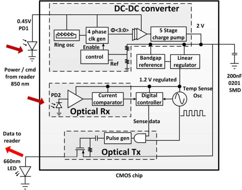
Figure 3. Architecture of the proposed sensing platform
