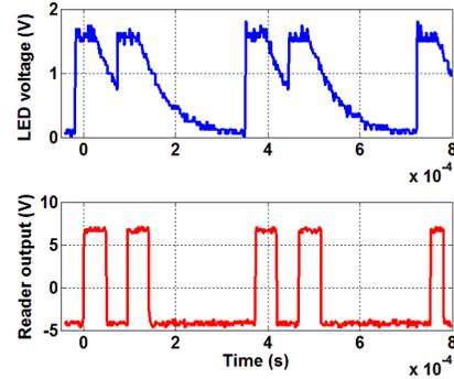
Figure 9. LED voltage at implant (Top) , Detected digital output at reader separated by pig skin from implant (bottom)
