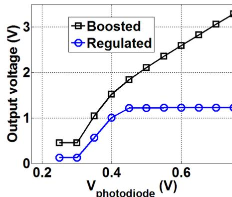
Figure 7. Measured power train performance
