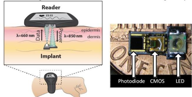
**Figure 1 . Proposed subcutaneous implant** powered sensing platform that achieves bidirectional optical telemetry.
