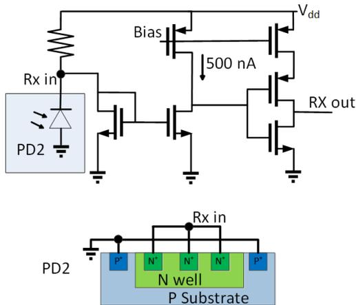
Figure 5. Fully integrated AFE and cross section of the on-chip photodiode
