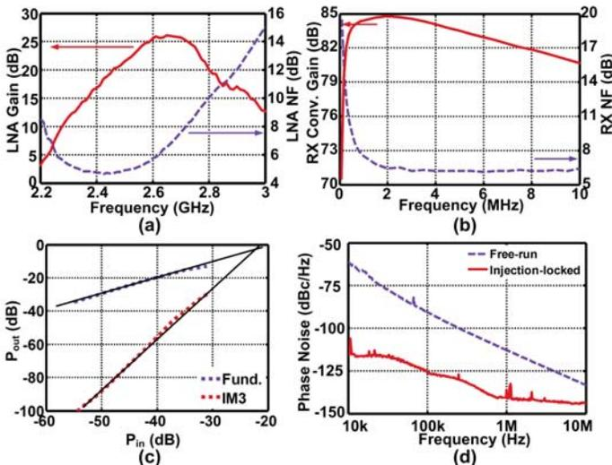
Figure 25.9.5: (a) LNA gain and NF; (b) receiver conversion gain and NF; (c) front-end IIP3; (d) VCO phase noise.
