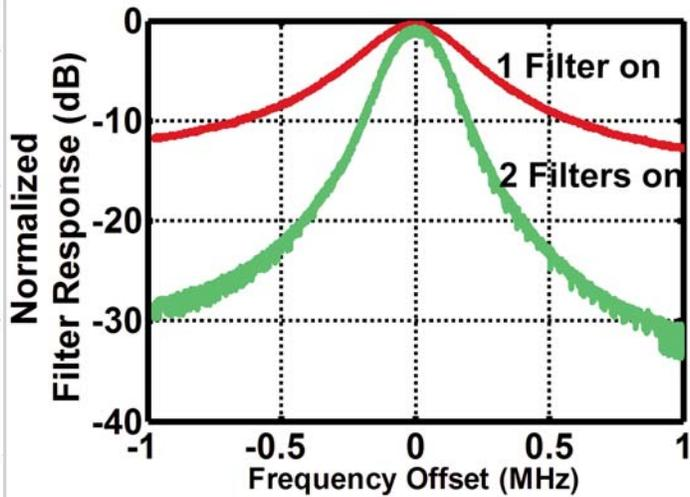
Figure 25.9.4: Measured IF frequency-translated filter response (normalized).
