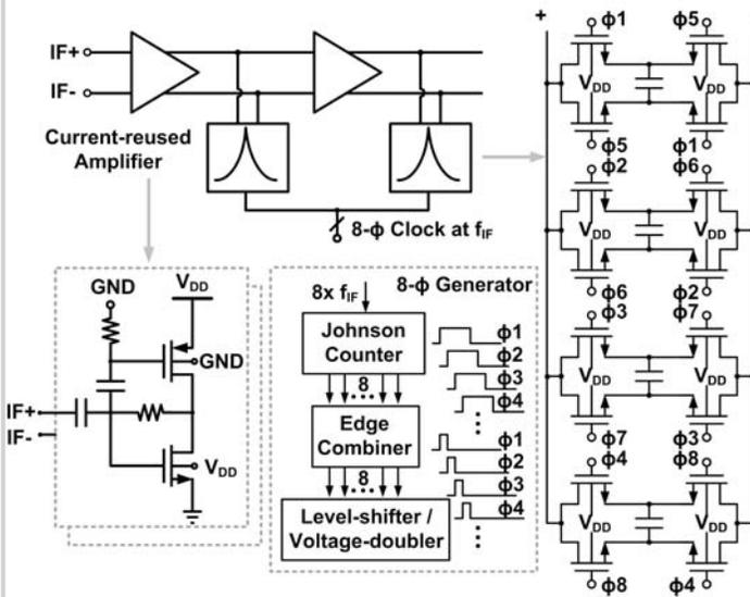
Figure 25.9.3: IF amplifier and frequency-translated filter schematic.
