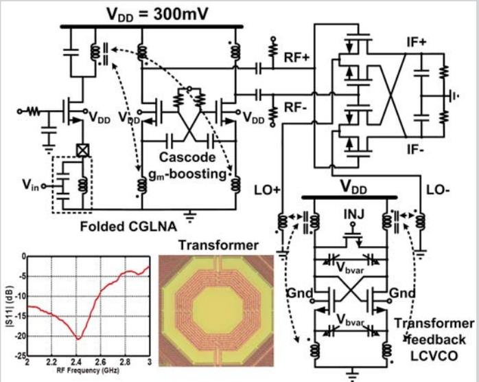
Figure 25.9.2: RF front-end (LNA, VCO, mixer) schematic (bias not shown).
