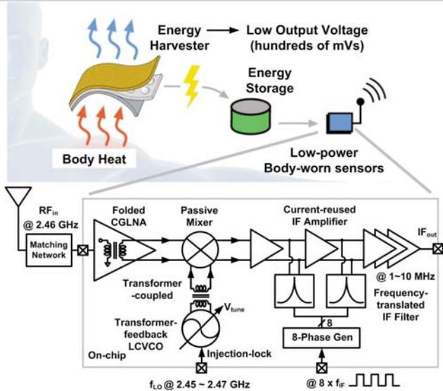
Figure 25.9.1: Proposed system block diagram.
