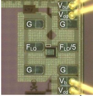
Figure 5. Die photo showing  $100\mu\text{m}^2$  ILFD and GSG RF input/output
