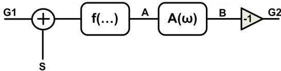
Figure 4. Analytical model for one stage of the ILFD
