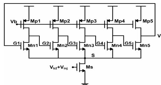
Figure 2. Proposed ILFD based on a 5-stage ring oscillator
