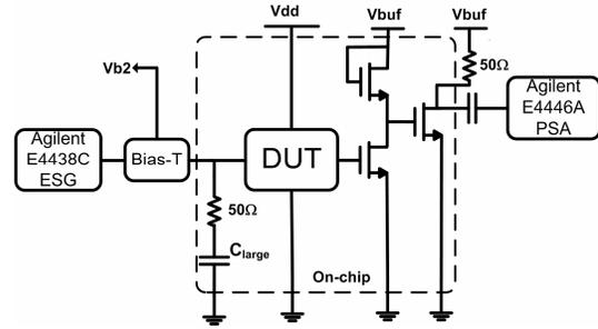
Figure 6. Experimental test setup. GSG wafer probes applied at the RF input
