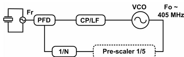
Figure 1. Architecture of ultra-low power MICS band frequency synthesizer
