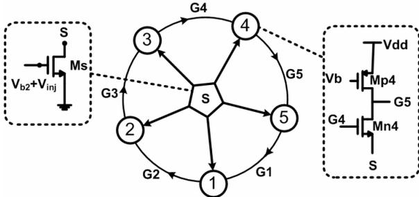
Figure 3. Conceptual drawing of the sequential injection at the 5<sup>th</sup> harmonic of the oscillator
