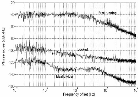
Figure 9. Phase noise performance of the ILFD compared with that of free running oscillation and the RF signal source alone
