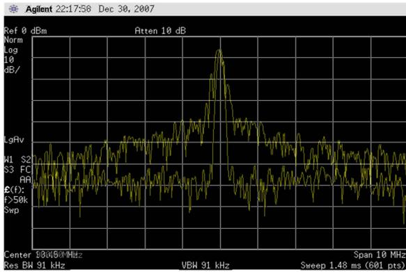
Figure 8. Free-running and locked spectra overlaid for comparison for an RF input of 500MHz
