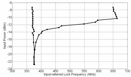
Figure 7. Frequency lock range of the ILFD
