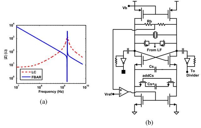
Fig. 3. (a) Tank impedance of FBAR and LC resonators. (b) The schematic of the VCO.
