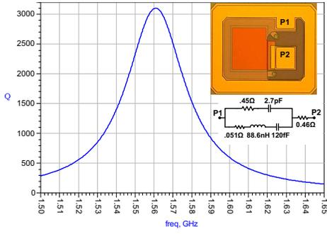
Fig. 2. Q vs. Frequency of an uncapped FBAR resonator.
