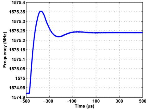
Fig. 8. PLL settling time measurement using an Agilent 5052B signal source analyzer.
