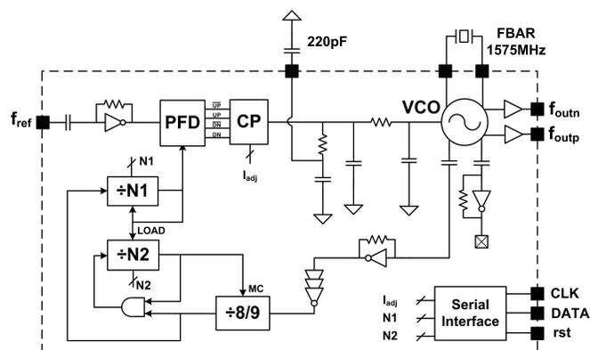
Fig. 1. The integer-N FBAR-based PLL architecture.
