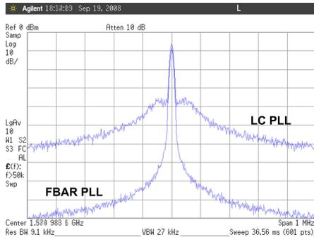
Fig. 10. Measured close-in frequency spectra of locked FBAR and LC PLLs.
