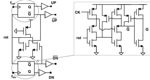
Fig. 4. Schematic of the phase frequency detector.
