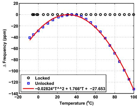
Fig. 11. Frequency vs. temperature stability measurements.
