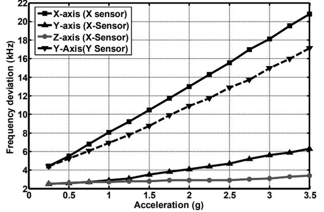
Fig. 7 Measured 3-axis of acceleration
