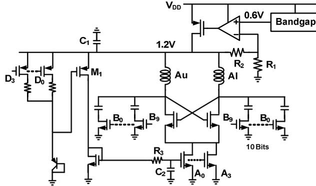
Fig. 3 Schematic of bondwire sensing oscillator
