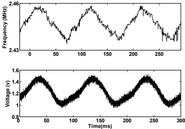
Fig. 9 Measured results of waveform at 10 Hz sinusoidal acceleration input with a 3g peak-to-peak amplitude (x-axis)
