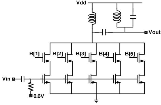
Fig.5 Schematic of driver amplifier
