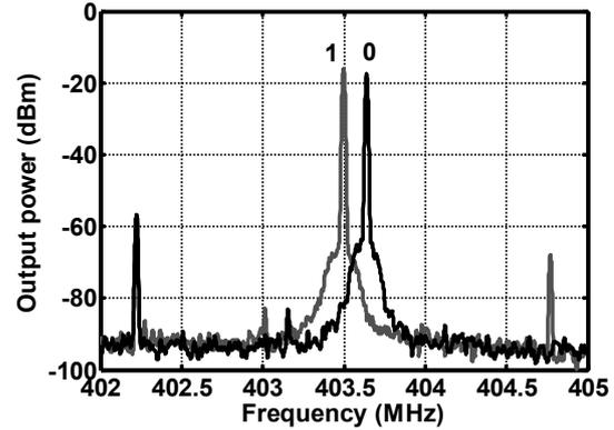
Fig. 10 Measured FSK transmitter output spectrum
