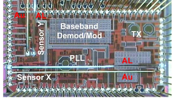
Fig. 6 Micrograph of the bondwire accelerometer
