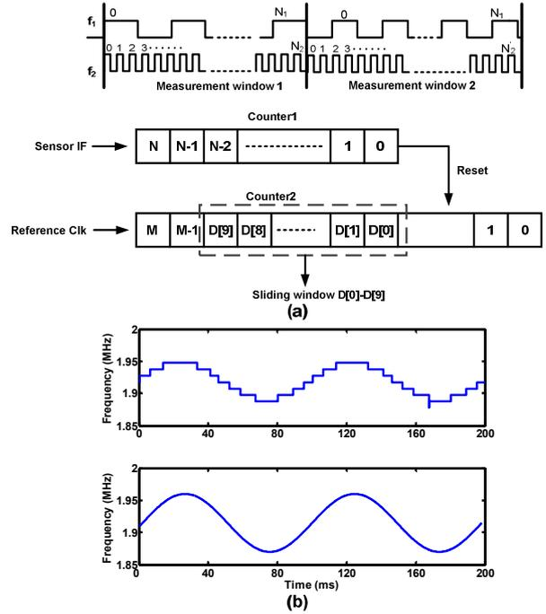
Fig. 4 Operation of frequency demodulator and measured digitalization result of a sinusoidal input
