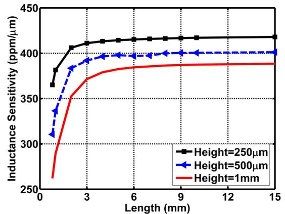
Fig. 1 FEM simulated results of inductive sensitivity (separation between two bondwires = 90  $\mu\text{m}$ )
