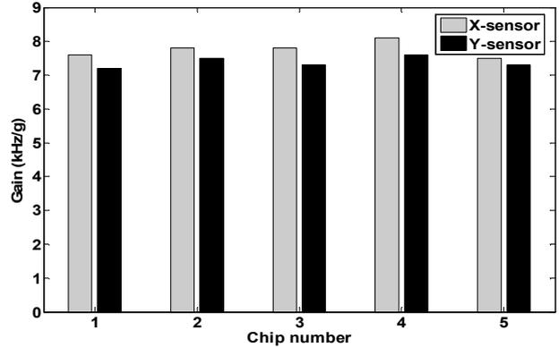
Fig. 8 Measured transducer gain of 5 chips
