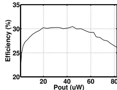
Fig. 9. Measured PA drain efficiency
