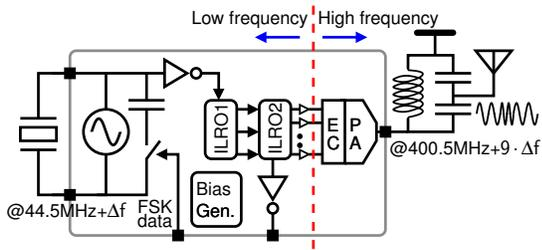
Fig. 2. Detailed block diagram of the proposed transmitter architecture for ultra-low power operation.
