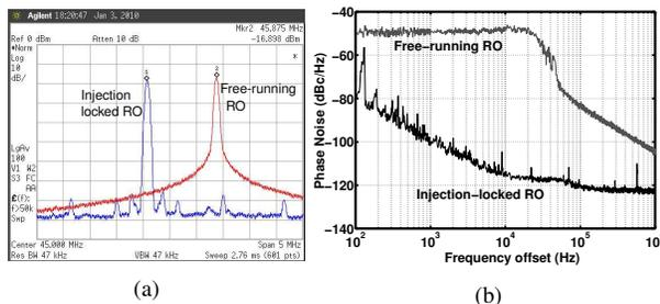
Fig. 6. (a) The spectrum and (b) the measured phase noise of the free running and the injection-locked ring oscillator.
