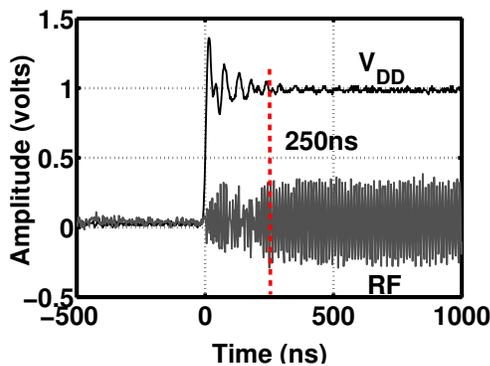
Fig. 12. A settling time  $< 250$  ns was measured.
