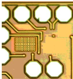
Fig. 11. The chip micrograph of the ultra-low power transmitter. The active area of the transmitter is  $\approx 200 \mu\text{m} \times 200 \mu\text{m}$ .
