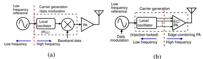
Fig. 1. (a) The conventional transmitter architecture (b) Proposed ultra-low power (ULP) transmitter architecture.
