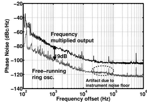
Fig. 8. Measured phase noise of the injection-locked LO and the frequency multiplied output using an Agilent E4446A spectrum analyzer.
