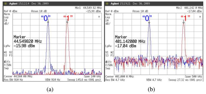
Fig. 7. (a) FSK modulated 44.5 MHz injection-locked ring oscillator.  $\Delta f_{RO} = 20$  kHz (b) FSK modulated frequency multiplied output at 400.5 MHz.  $\Delta f_{RO} = 180$  kHz
