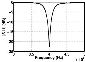
Fig. 10. Measured input return loss.  $|S_{11}| < -10$  dB.
