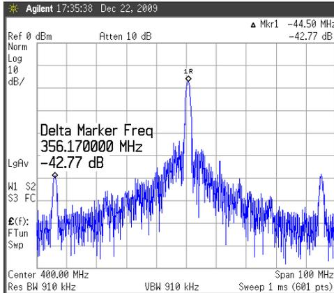
Fig. 5. Measured carrier-to-spur ratio of 42.77 dB was achieved.
