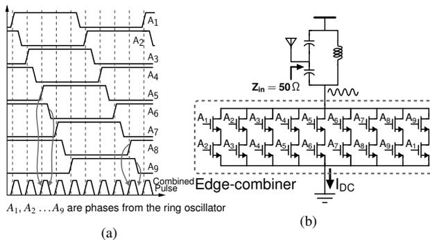
Fig. 3. (a) The principle of edge-combining (b) Schematic of the edge-combiner.
