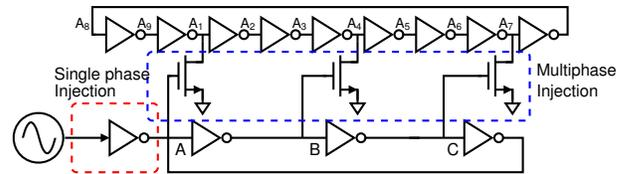
Fig. 4. Schematic of the two-stage multi-phase injection-locked ring oscillator.
