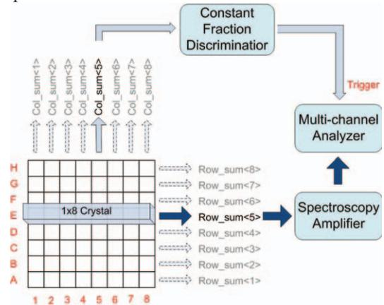
Fig. 7 Experiment setup for energy resolution measurement
