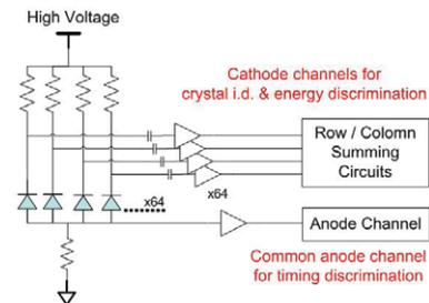
Fig. 4. Biasing circuit for simultaneous signals pick-off on the common anode and individual cathodes
