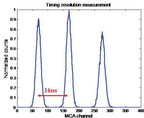
Fig. 11. Timing resolution measurement result
