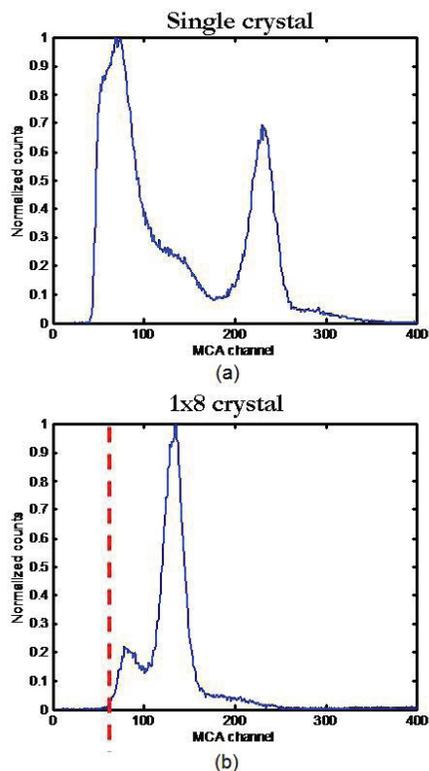
Fig. 8 Energy spectra from cathode channels (a) with single crystal (b) with 1x8 crystal array
