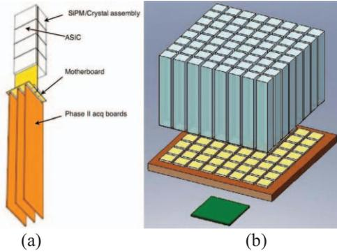
Fig. 2 (a) Architecture of the proposed detector module (b) Detector assembly
