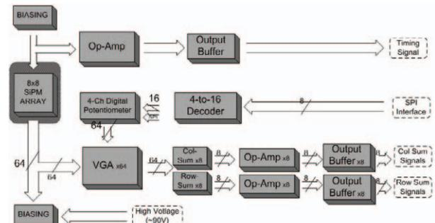
Fig. 3. Block Diagram of the readout electronics.
