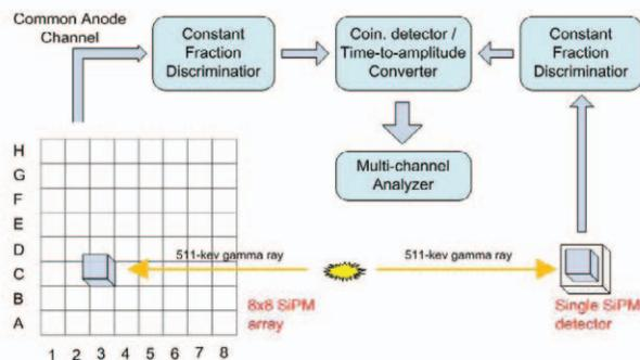
Fig. 10 Experiment setup for timing resolution measurement
