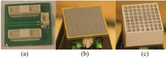
Fig. 1(a) Connectors of the 8x8 SiPM array (b) SiPM elements (c) 8x8 LFS crystal array
