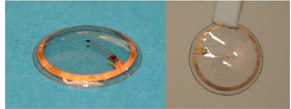
Fig. 14. Unlit and wirelessly lit active lens assembly.
