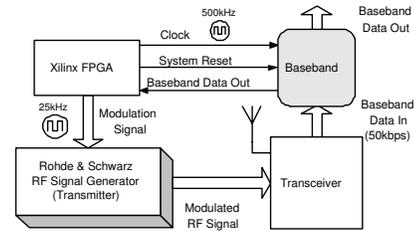
Fig. 6. Measurement setup
