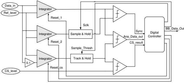
Fig. 3. Block diagram of the baseband silicon implementation
