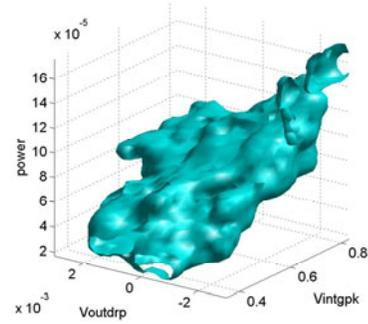
Fig. 5. Integrator performance space projection. The volume shows a feasible range of the integrator performance in terms of output voltage droop, integration peak level, and power consumption
