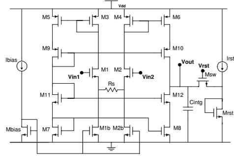
Fig. 4. Schematic of  $G_m - C$  integrator
