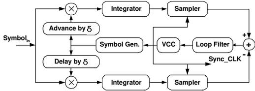
Fig. 1. Block diagram of Early-Late Gate synchronizer
