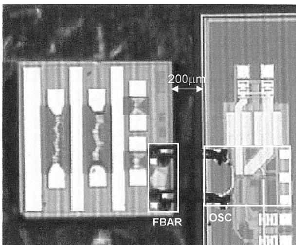
Fig. 4. Photograph of the CMOS oscillator wire bonded to the FBAR resonator.
