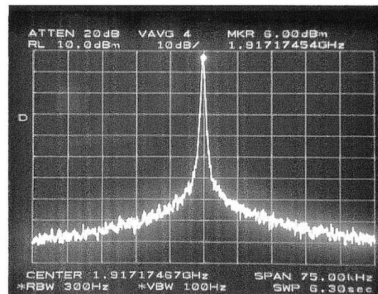
Fig. 5. Oscillator frequency spectrum.
