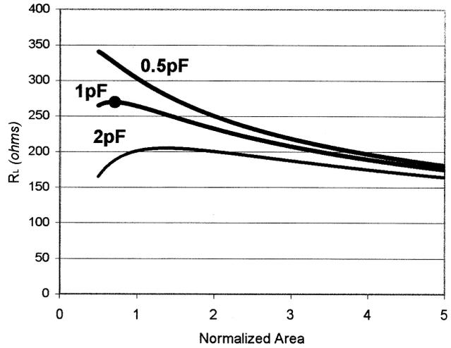
Fig. 2. Optimization of resonator area for three values of  $C_1 = C_2$ . The design point is indicated by the curve marker.
