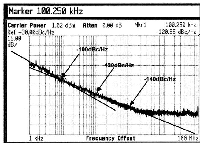
Fig. 6. Measured phase noise of the oscillator.
