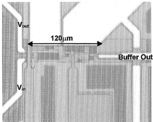
Fig. 3. Die photograph of CMOS oscillator core.
