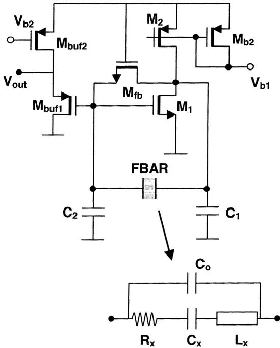
Fig. 1. Simplified oscillator schematic and FBAR resonator circuit equivalent model.
