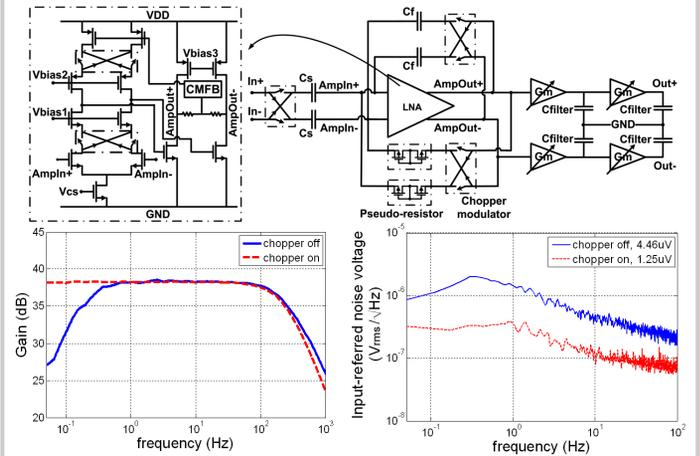
Figure 2.8.4: LNA schematic, gain and noise versus frequency.
