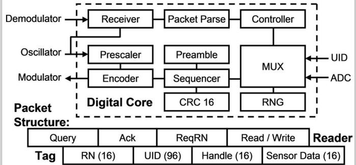
Figure 2.8.2: Digital core and packet structure.
