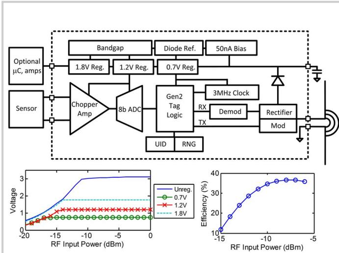
Figure 2.8.1: System architecture and performance.
