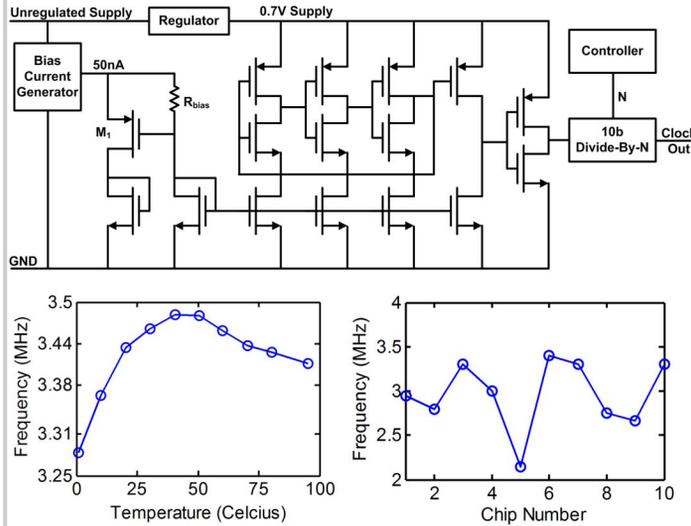
Figure 2.8.3: Oscillator schematic and performance.
