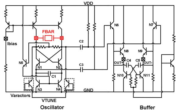
Figure 3: Schematic of the oscillator and buffer.
