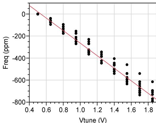
**Figure 7: Measured tuning curve of ZDR oscillator.**
