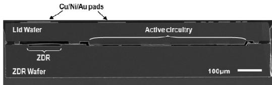
Figure 2: Cross-section SEM of FBAR/bipolar process showing full finished die.
