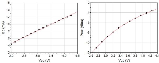
**Figure 4: Measured oscillator current (left) and output power (right).**
