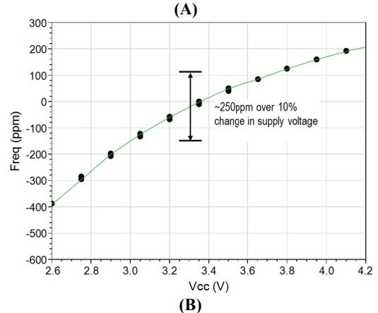
**Figure 5: (A) Measured oscillator frequency drift as a function of temperature. (B) Measured oscillator frequency variation as a function of supply voltage.**
