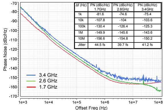
**Figure 6: Phase noise of the oscillators with 3 resonators of 1.7, 2.6, and 3.4 GHz respectively, measured with an Agilent 5052 signal source analyzer.**
