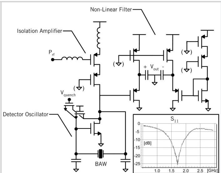
Figure 21.4.2: Receiver front-end schematic and measured input matching.
