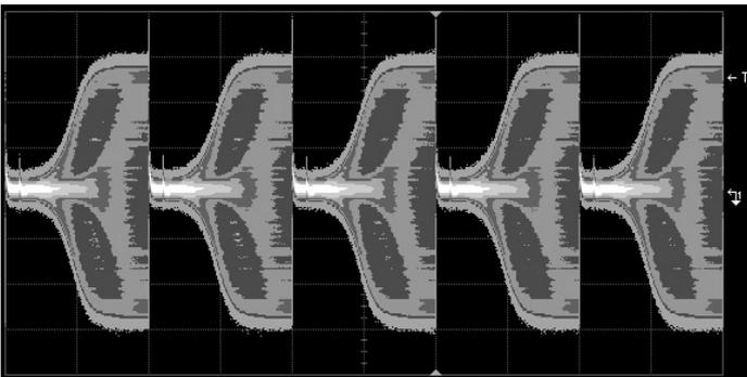
Figure 21.4.3: Detector oscillator eye diagram for -80dBm input.
