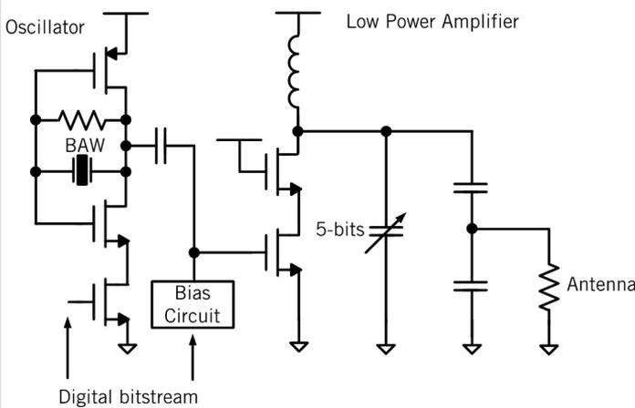
Figure 21.4.5: Transmitter Schematic.
