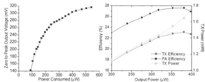
Figure 21.4.6: Oscillator and transmitter performance curves.
