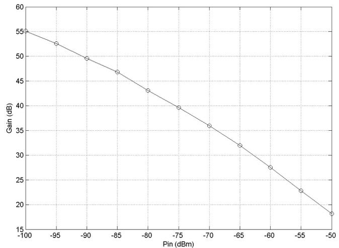
Figure 21.4.4: Logarithmic gain response of the receiver.
