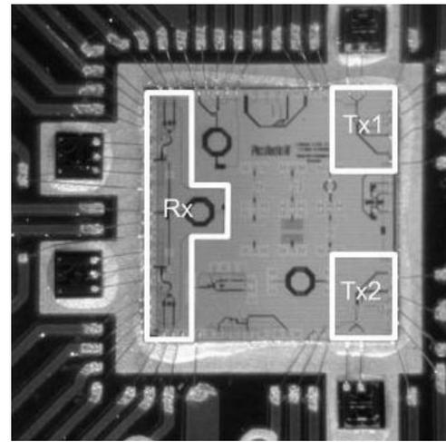
Fig. 7 Transceiver Photograph
