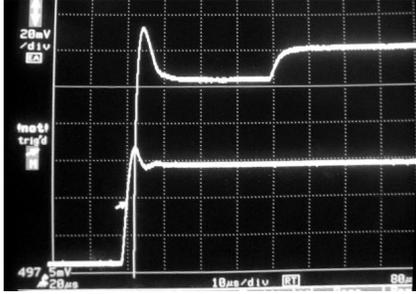
Fig. 10 Receiver Start-Up ( $10\mu\text{s}/\text{div}$ )
