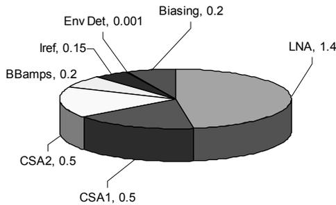
Fig. 11 Receive Current Consumption Breakdown (mA)
