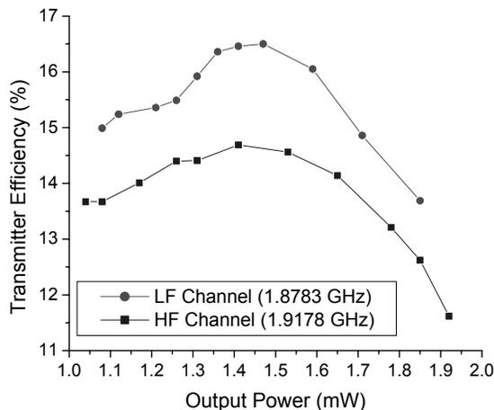
Fig. 12 Transmitter efficiency versus output power
