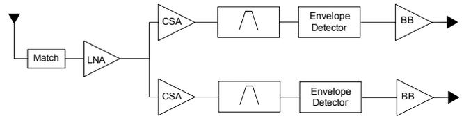
Fig. 1 Receiver Architecture
