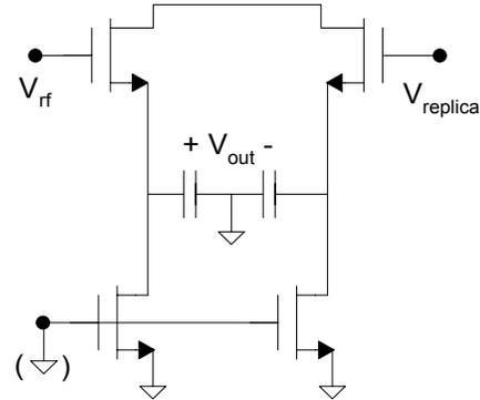
Fig. 4 Envelope Detector Schematic
