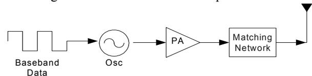
Fig. 5 Direct modulation transmitter architecture
