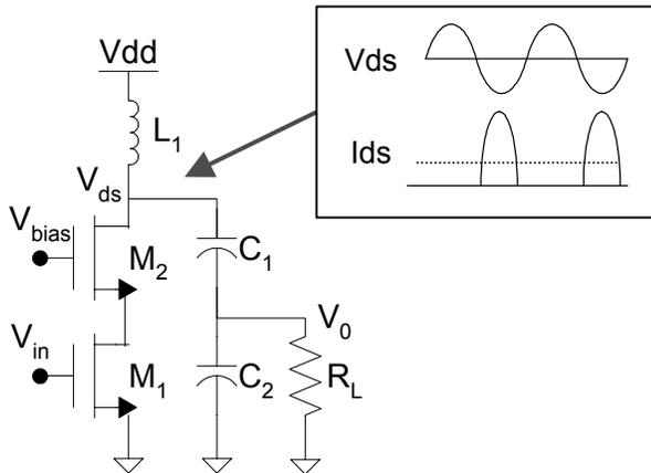
Fig. 6 Schematic of the low-power amplifier
