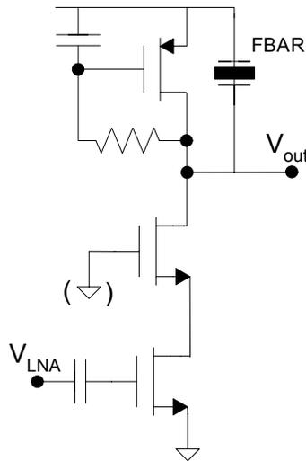
Fig. 3 Channel Select Amplifier Schematic
