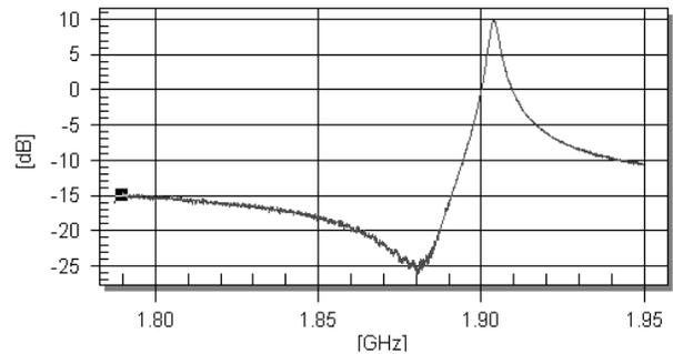
Fig. 8 Measured S21 of Channel Select Amplifier
